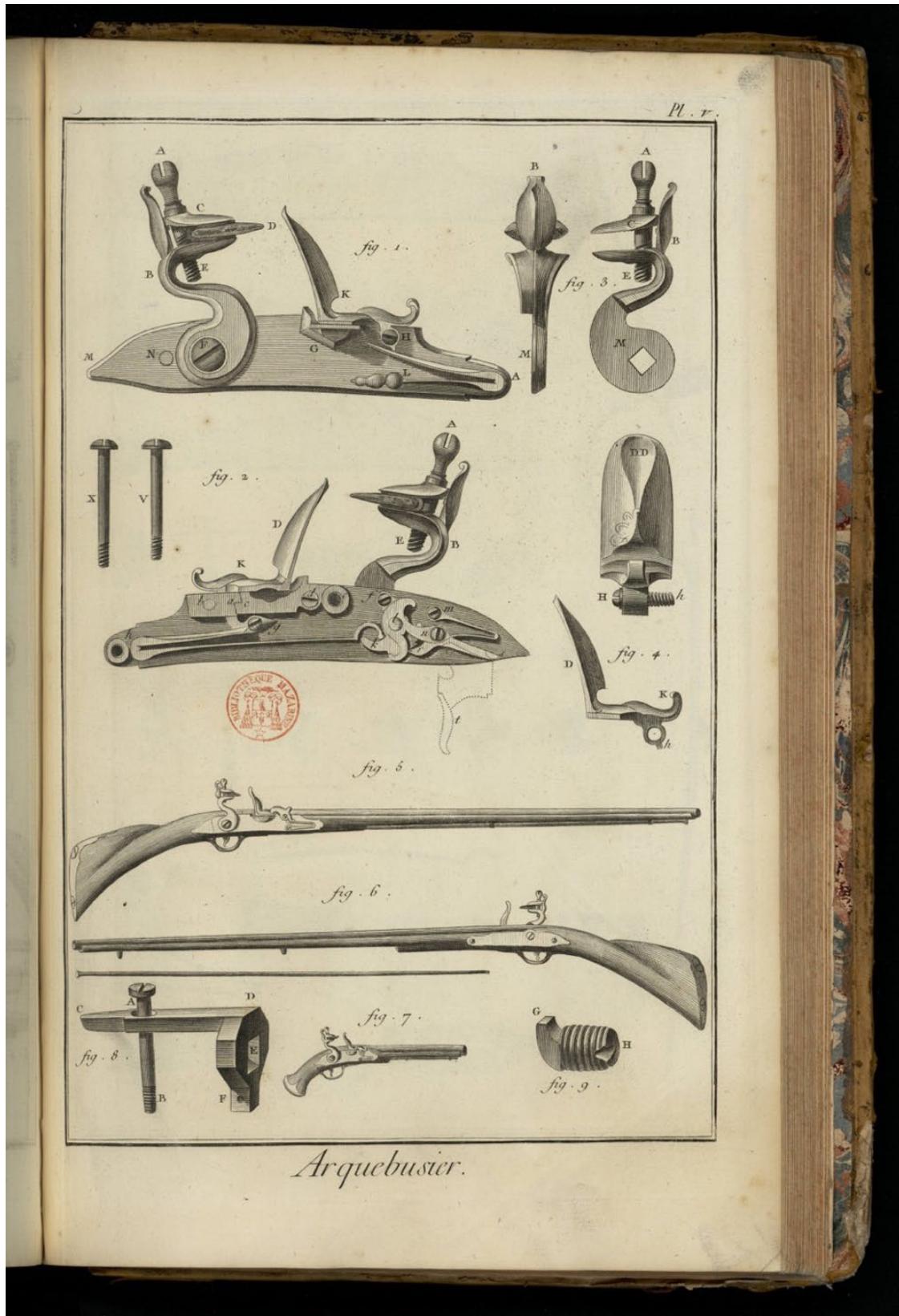
Views of a mid-18th-century French flintlock mechanism, lock screws, cock/hammer, frizzen/battery, muskets, false breech, pistol, and breech plug, from Diderot's L'encyclopédie, ou Dictionnaire Raisonné des Sciences, des Arts et des Métiers: Recueil de Planches sur les Sciences et les Arts (Paris, 1770), vol. 1, Plate V. Note the outline of the trigger, below, Exhibit C
