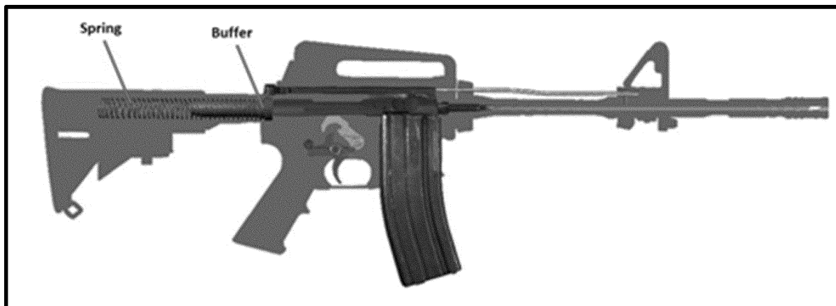
Internal function of an AR-type rifle
